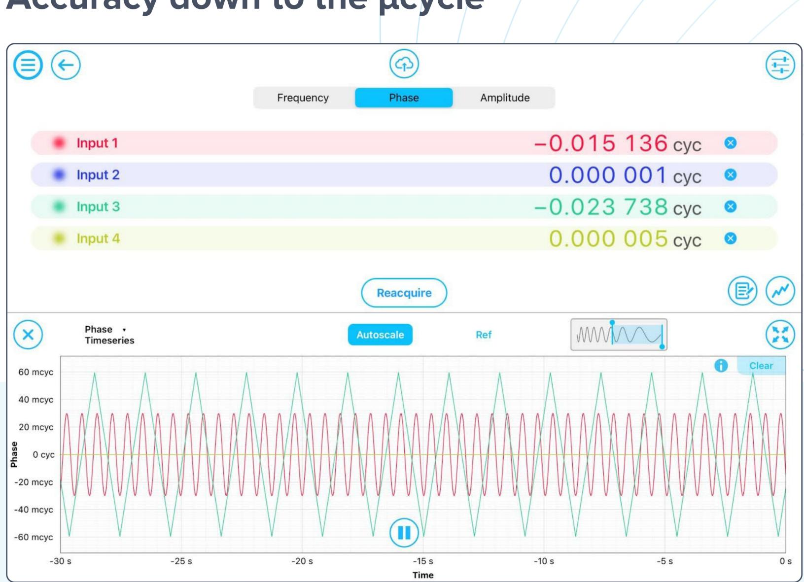
It's important that your measurement device has enough precision to get meaningful results. Here, we're using the Moku Phasemeter to measure phase with part-per-million accuracy.
